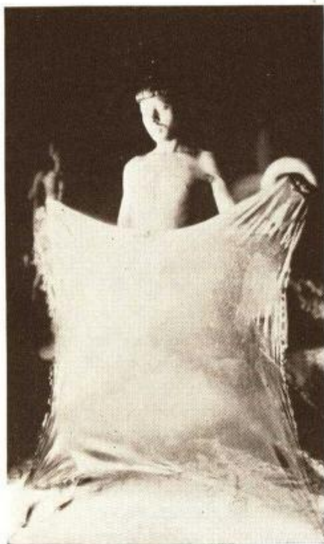
Cooled molten Shellac stretched into thin sheets prior to breaking into flakes
